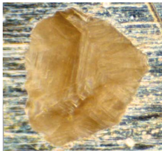
Fig. 8 The great deal of slippage and twins form during \text{Mg} \rightarrow \text{MgH}_2 phase transformation
